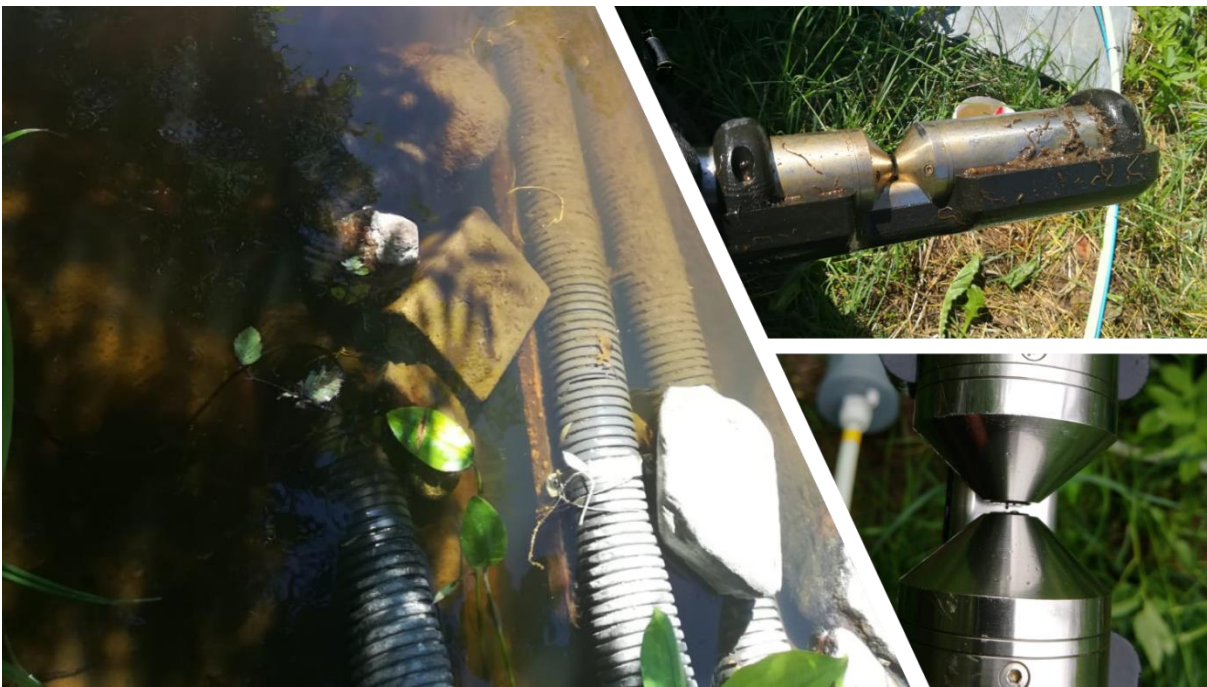
Figure 13. In the summer of 2020, the water level dropped and a lot of light, brown particles were observed in water. The sensor became dirty and the measurements may therefore be incorrect. In such a situation, frequent cleaning of the sensor is necessary.
